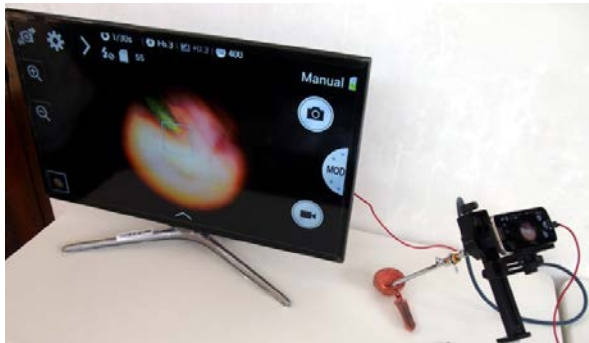
Figure 1: Setup of wired “screen mirroring” connecting Smartphone with LCD monitor using red MHL cable during simulated cystoscopy using bladder-urethra model.
