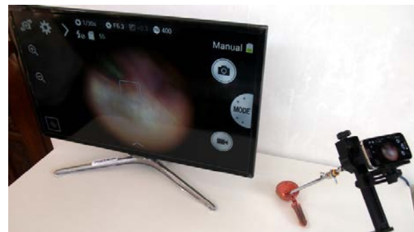
Figure 2: Setup of wireless “screen mirroring” with compatible LCD monitor and Android Smartphone during simulated video cystoscopy using bladder-urethra model.
