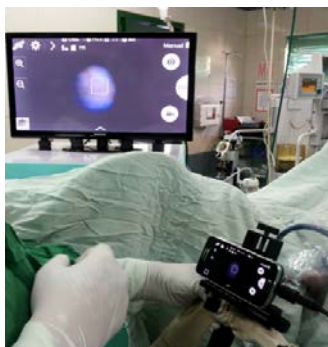
Figure 3: Screw-in universal digiscoping adapter to phone after MHL cable connection.
