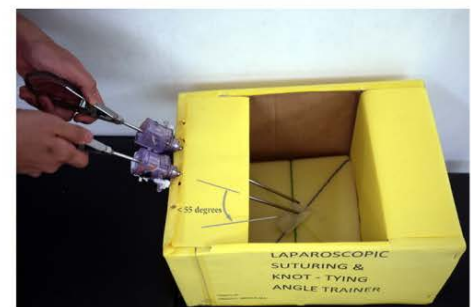
Figure 3: The angle between each straight instrument (telescope, needle holder, and grasper) and the horizontal line is less than 55 degrees.
