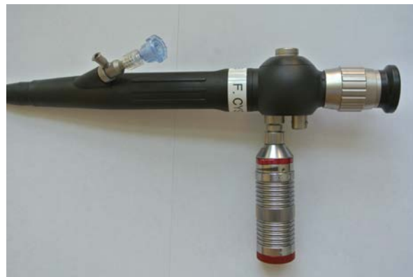
LED light source attached to cystoscope
