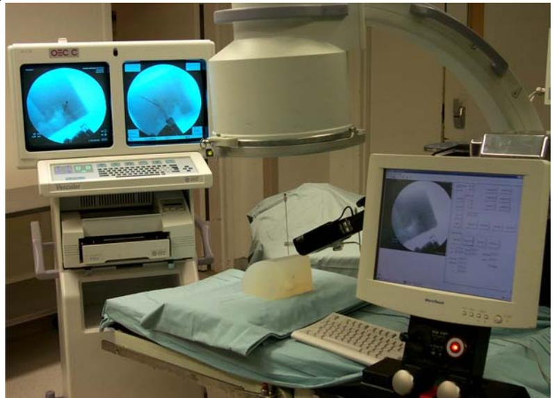
Figure 1: AcuBot in C-Arm guided needle insertion experiments
